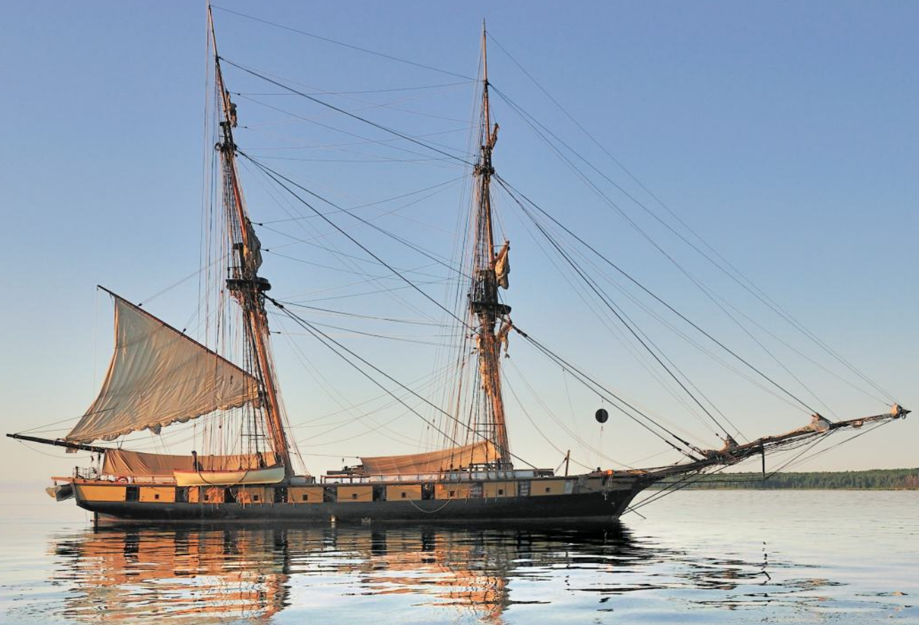
THE NIAGARA AT THE MOUTH OF PARADISE BAY & THE TWO LIGHTS OF SOUTH FOX ISLAND SPARRED LENGTH: 198' · LWL: 110' 8" · BEAM: 32' · DRAFT: 10' 6" · DISPLACEMENT: 297 LONG TONS · MAINMAST: 118'
